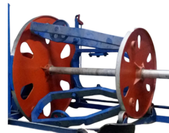
4. CABLE CORE LAYING UP MACHINE
