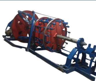
6. ARMOURING CUM CORE LAYING MACHINE
